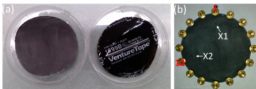
Figure 1. (a) A thin plastic tape with carbon nanotube coated paper to enhance physical durability, front (left) and back (right) of the CNCP ( d = 7 cm). (b) CNCP fixed with 16 electrodes, located around the CNCP boundary. Numbering of the electrodes is clockwise starting from top (1 in red colored). The closest distance between two adjacent electrodes is 0.6 mm. Two intentional damages (X1 and X2) are located at 1 cm from the CNCP periphery near electrode 1 and 12.
